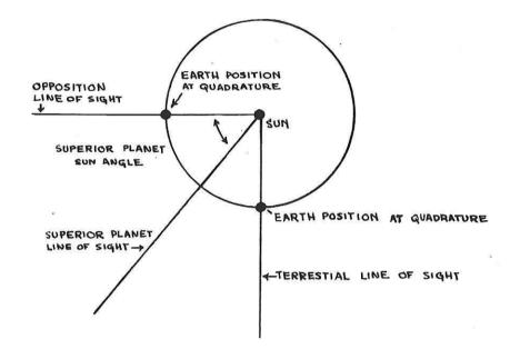
4. To determine the exact location of the superior planet on the superior planet line of sight, construct a tangent perpendicular to the terrestrial line of sight at the earth position at quadrature. Extend the perpendicular until it intersects the superior planet line of sight. This point of intersection is the position of the superior planet.
