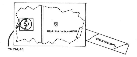
Directions for use: The thermometer must be in the light beam produced through the opening in the partition. As one student uses the calibrated rheostat to reduce the bulb in brilliance, another student records temperature changes as shown on the thermometer, while a third student looks through the spectroscope and records color bands.
