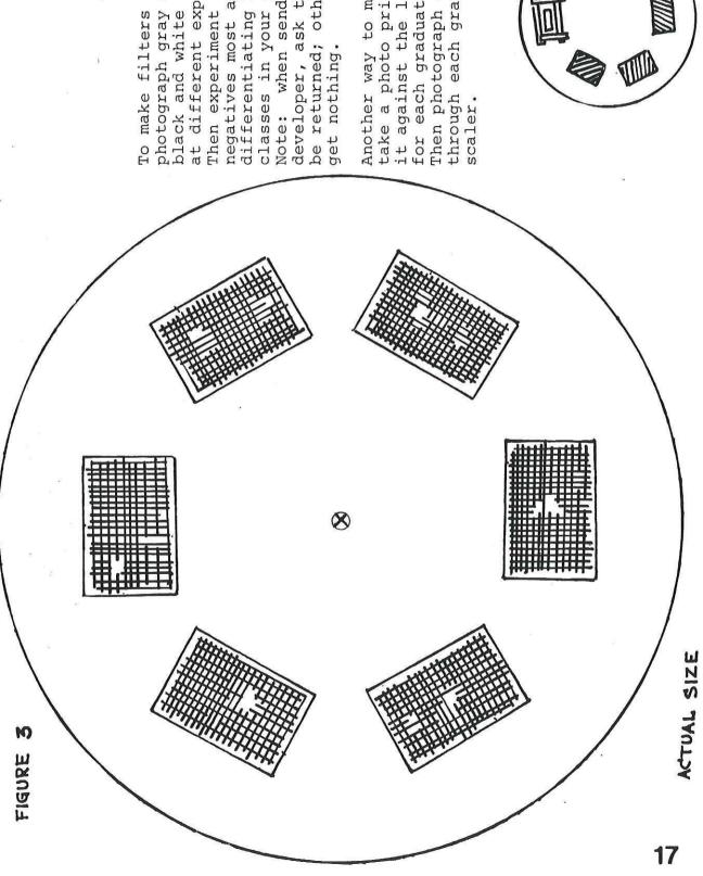
To make filters (negatives), photograph gray cardboard using black and white film (35 mm slides) at different exposures (F stops). Then experiment selecting the negatives most appropriate for differentiating between magnitude classes in your planetarium sky. Note: when sending film to developer, ask that all negatives be returned; otherwise you will get nothing.
