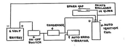
Note: to vary intensity of source the distance between the points within the transmitter may be adjusted.
