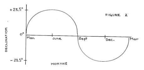
The correction factor, declination, may be easily determined as shown above after plotting the annual path of the sun with respect to the celestial equator. (For the development, students can provide declination data from their planetarium data sheets.)
