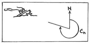
b. Bearing is also measured clockwise from north. Below the bearing of a ship at A headed toward B is the angle measured clockwise from the north line and is the angle B/A (B/A means B relative to A). Likewise the bearing of a ship at A headed toward B is the angle A/B.
