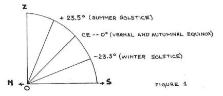
The distance from the celestial equator to the zenith of the observer is equal to the observer's latitude. Therefore, angle ZOCE = latitude. But the sun is located at CE only on dates of the vernal and autumnal equinoxes. At other times it shifts from CE  $(0^{\circ})$  to +23.5° on June 21 to -23.5° on December 21. To determine latitude by the sun, you must return the sun mathematically to the equator by a correction factor-the sun's declination.
