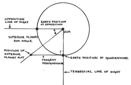
5. Continue the above procedure for each position of the superior planet until all points are plotted. Then connect the plotted superior planet points with a continuous curve which completes the orbit of the planet.
