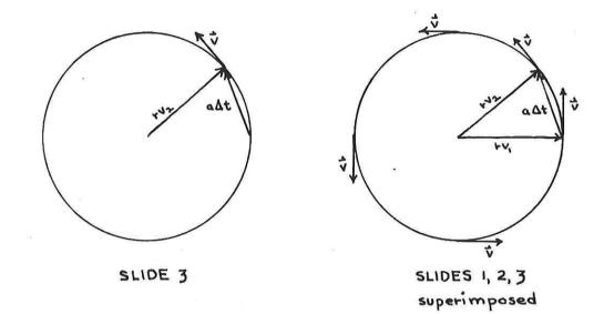
Discuss the motion of the head of the velocity vector, leading students to discover that this is an acceleration vector ( $a\Delta t$ ). Then discuss the angular relation between the radius vector and the acceleration vector. You can use your planetarium pointer to show that the radius vector is directed outward, the acceleration vector directed inward.
