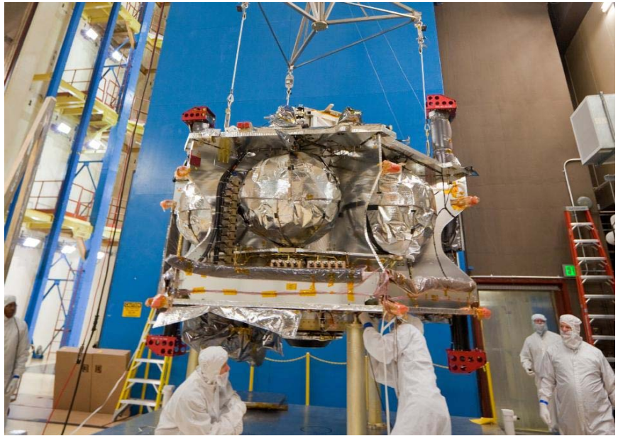
Technicians lift NASA's Juno spacecraft onto a dolly prior to the start of a round of acoustical testing. Image Credit: NASA/JPL-Caltech/LMSS
